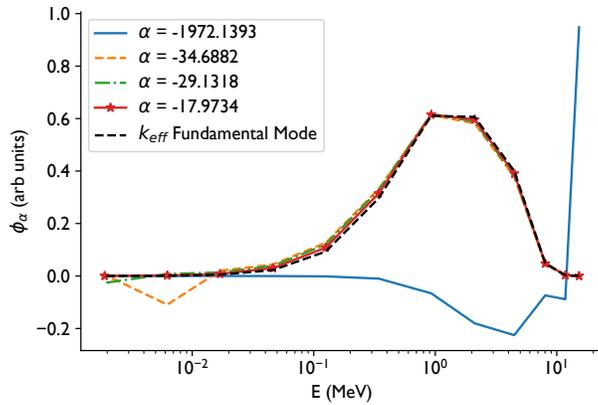
Figure 1: Comparison of scalar flux for the fundamental  $k$  eigenmode with 4  $\alpha$  eigenmodes for the subcritical sphere.
