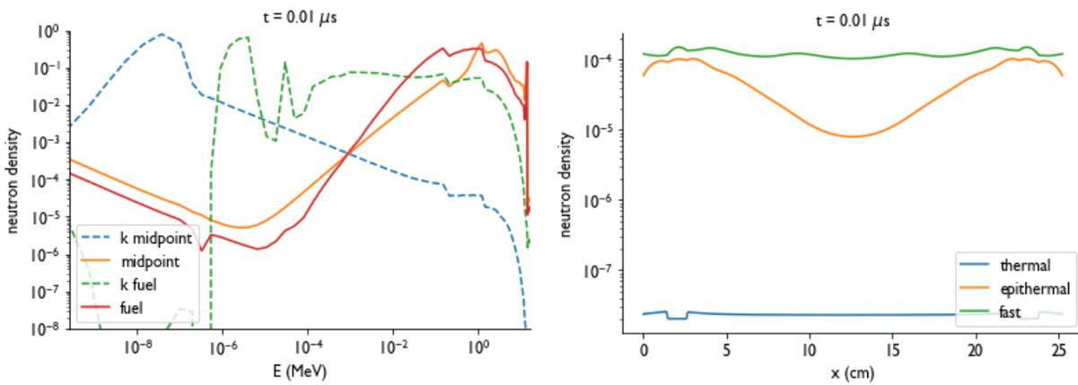
Figure 2: Spatial profile for neutron density and spectrum the center of the fuel and at the midpoint of the problem at  $0.01 \mu s$ .
