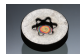
Here is a picture of the americium from inside a smoke detector. The colorful part in the middle is the americium: the americium is smaller than a grain of sand.
