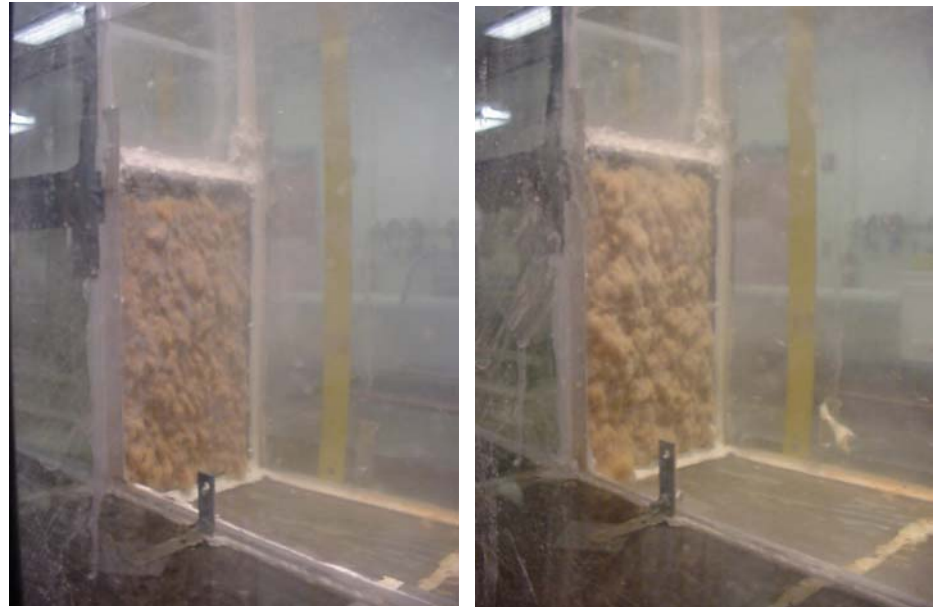
Pictures from insulation debris clogging experiments (NUREG/CR-6762, Vol. 1)
