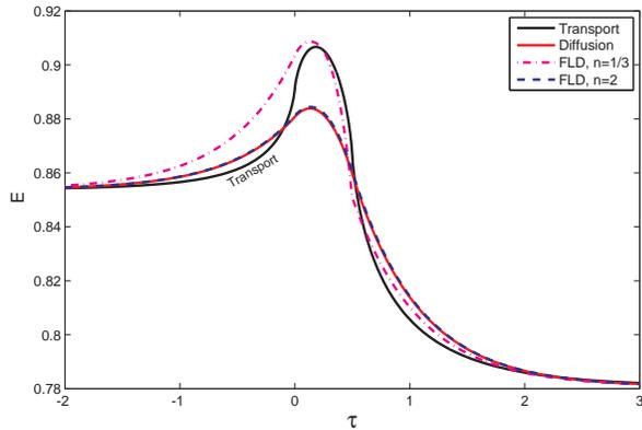
Fig. 4: Transport and diffusion solutions for a thick cooling layer.
