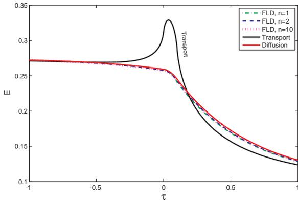
Fig. 1: Energy density solutions using various integer  $n$  values when applied to a temperature profile with a thin cooling layer.
