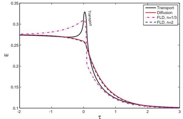
Fig. 3: Transport and diffusion solutions for a thin cooling layer.
